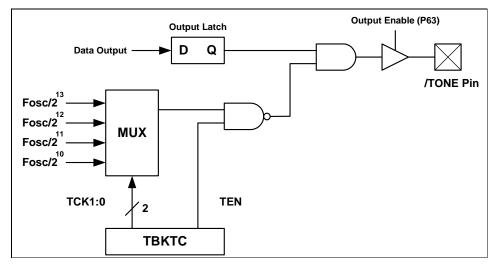
Fig. 5-6 Tone Output Pin Configuration
